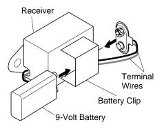
Figure 28 - Attaching Battery to Receiver
